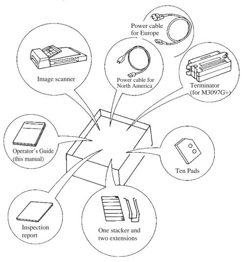
Figure 2.1 Received components
